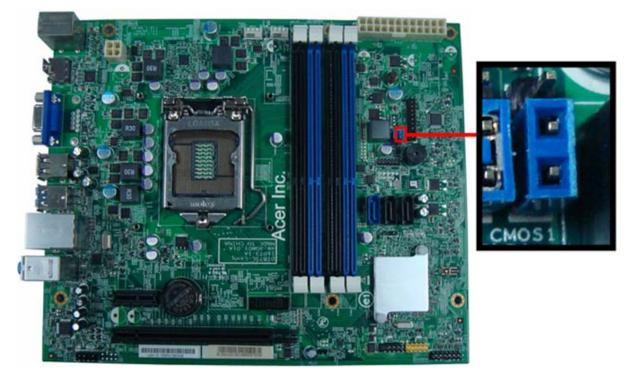
The following table shows the settings of the 3-pin SW1 jumper. Place the jumper cap on pins 1 and 2 to close or short the jumper. Place the jumper cap on pins 2 and 3 to open or clear CMOS.
